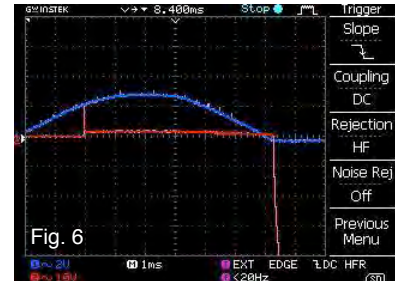
Fig. 6: With a NOsparc arc suppressor across the relay contacts, the break arc is immediately suppressed and held for the 7ms until the current approaches the zero-crossing.
