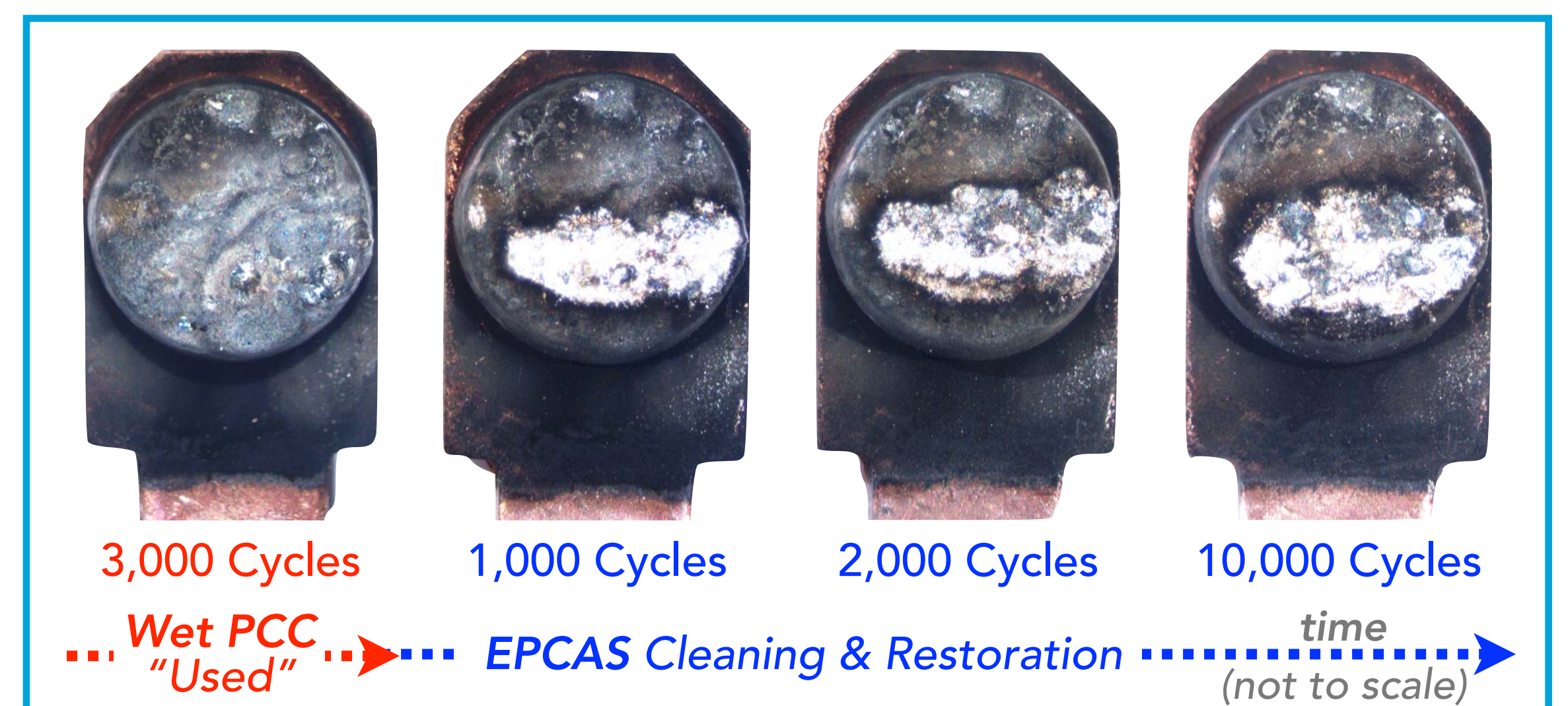
Figure III: Failed Contacts from Wet PCC after Restoration by EPCAS Cycles
